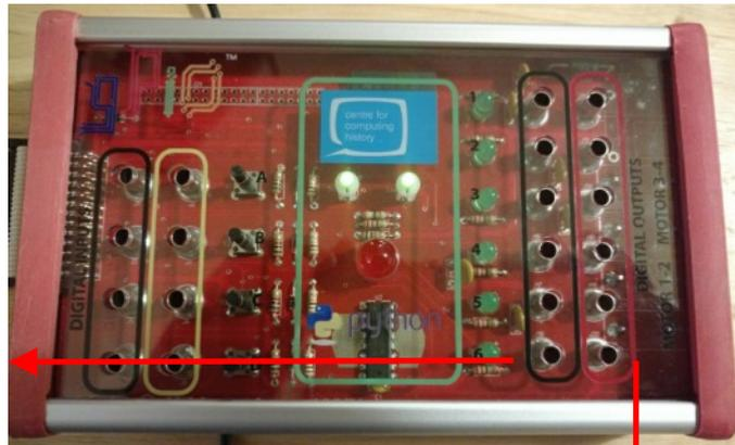
Make sure you connect the banana plug with the **red (positive) wire** inserted into the **output 1** slot with the '**red**' box around it. Similarly, the banana plug with the **black (negative) wire** inserted goes into the **output 1** slot with the '**black**' box around it.
