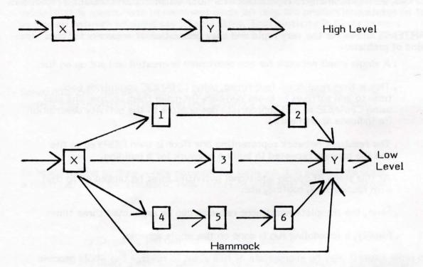
The usual method of doing this involves identifying nodes in the high level network with specific nodes in the lower level network by using the same node number (not absolutely essential, since they can be "translated" via an intermediate dataset if it's desired to use a different node labelling system in the two networks). In addition, each activity in the higher network is represented by a hammock in the lower one.
