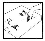
Holding the cartridge tilted with the plastic knob uppermost and to the left, engage the two catches on the left and right sides frame hooks on the printer. Then press down the front of the cartridge and engage the side tabs.
