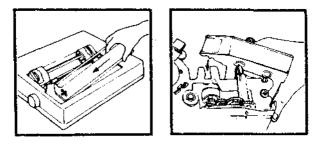
Tighten the ribbon once more, ensuring that it slips in front of the printer head, but behind the metal shield.
