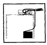
Pull the paper release lever towards you, to the RELEASE position.
