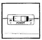
9 The POWER, READY, and ON LINE lights will come on. If the PAPER OUT light comes on, check that the paper is properly installed.
