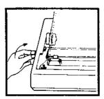
Adjust the paper so that a perforation between sheets is positioned slightly above the top of the ribbon.
