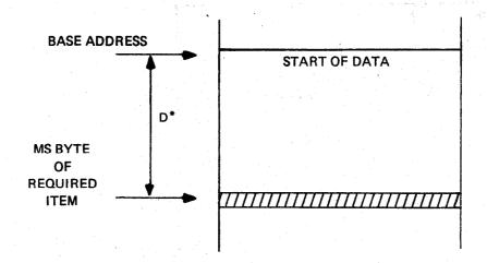
The displacement field is scaled as for format A1 and the 7 bits of this field may be used to access one of 128 items (bytes, halfwords, words, or double words) in the area defined by a base register.
