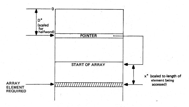
This format is used to access global arrays, the 6 bits of the displacement field allowing up to 64 array pointers to be used.
