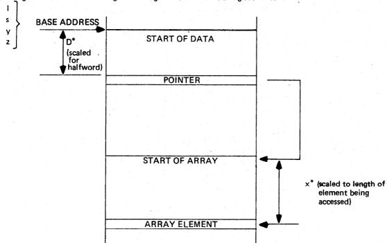
The 5 bit displacement field may be used to access one of 32 array pointers in an area of store defined by a base register.
