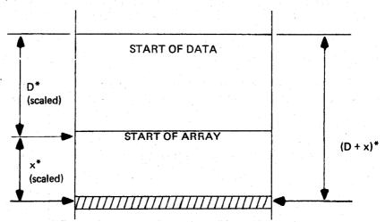
The displacement field and x are scaled according to the length of the item to be accessed from store. The four bits of displacement field enable 16 items (bytes halfwords, words or doublewords) to be accessed from store in the area defined by a base register and the index register x.
