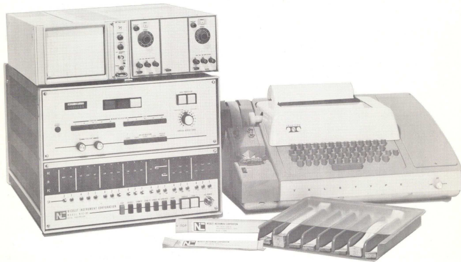
Figure 1: The minimal NIC-80 configuration 6 as purchased by Lancaster. It consists of the NIC-80 itself with 8K of internal memory, plus a high-resolution Tektronix CRT display for data (on top), a set of paper tapes with Nicolet programmes (front), and an ASR 33 Teletype (right). Later, we added a third 4K stack of ferrite core memory and NIC-298 (floppy) and NIC-294 (Diablo) disk drives. We also replaced the Teletype with a VDU together with an optical tape reader and fast punch.
